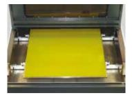
The processor includes a self-adhesive holder for positioning the plate, integrated heating and cooling device for solvent temperature control and automatic replenishment.
